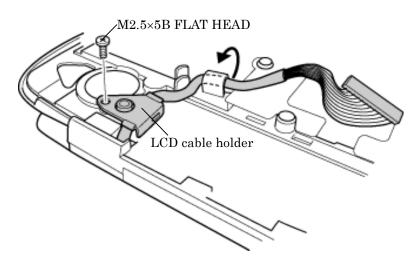
Figure 4-43 Removing the LCD cable holder
